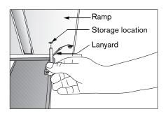
Diagram 4: Store the locking pin under the ramp
